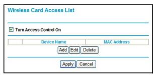
The Turn Access Control On check box is not selected so that any computer configured with the correct wireless network name (SSID) and passphrase to access the network.
